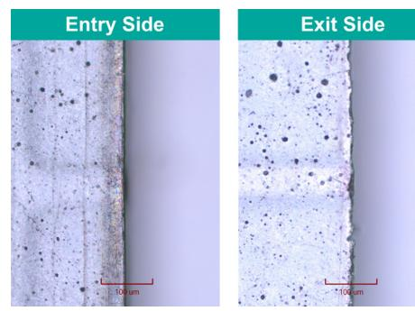
■ Figure 4. Cutting results for the 200 µm thick SiP substrate using a green USP laser operating at 20 W. These microscope photos show the entry and exit sides of the cut around the copper trace. There is a clear improvement over the results obtained at full power operation. Specifically, the HAZ surrounding the copper has been essentially eliminated. The speed in this case can be increased significantly by using a higher power ps UV laser and splitting the beam.
