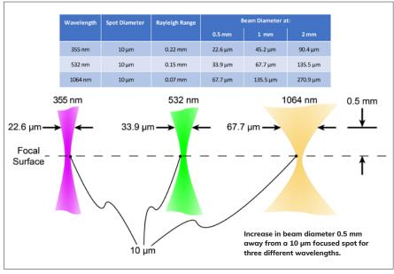
■ Shorter wavelengths have a longer depth-of-focus. If three different lasers are all focused to a 10 µm spot, they will have each spread a different amount 0.5 mm away from the focal plane.
