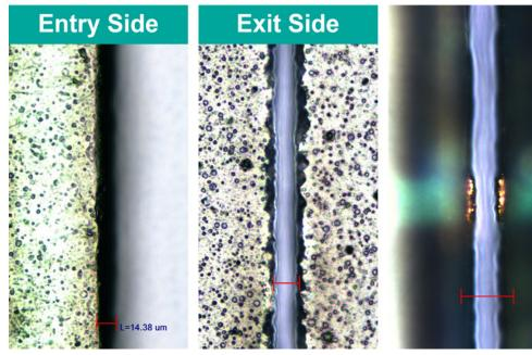
■ Figure 1. Cutting results for the 250 µm thick SiP substrate using a green nanosecond laser. These microscope photos show the entry and exit sides of the cut, plus the cut through the copper trace.
