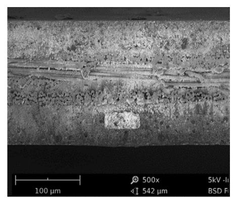
■ Figure 5. Sidewall view of a 200 µm thick SiP substrate cut with 20 W of green USP laser power. The substrate demonstrates excellent quality, particularly within the glass fiber weave and adjacent to the buried copper trace.
