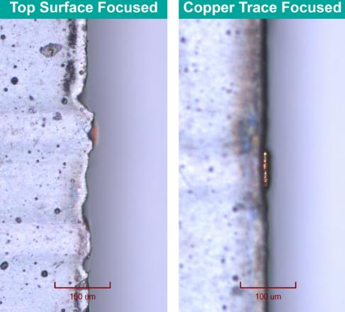
Figure 3. Cutting results for the 200 µm thick SiP substrate using a green USP laser operating at 40 W. These microscope photos both show the entry side of the cut, with one focused to emphasize the slightly protruding edge of the copper trace. While cut quality is good, there is some HAZ around the copper trace.
