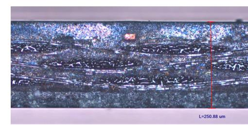
■ Figure 2. This sidewall view of a green nanosecond laser-cut, 250 µm thick SiP substrate demonstrates good quality, with minimal glass fiber melting and no HAZ adjacent to the buried copper trace.
